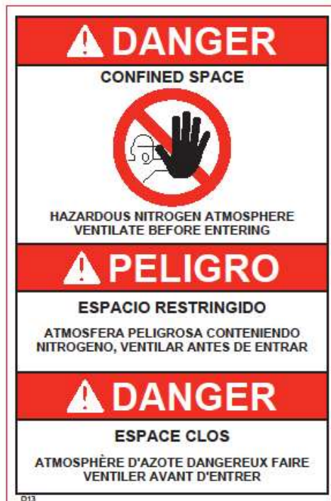
Figure 1 – Warning Label - Confined Space (applied to all transformer tanks)
