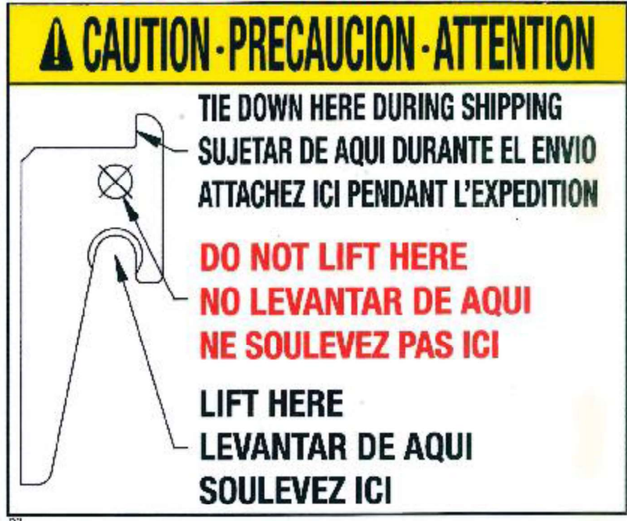
Figure 4 – Caution Label – Lift and Tie down Instruction (applied to all transformer tanks)
